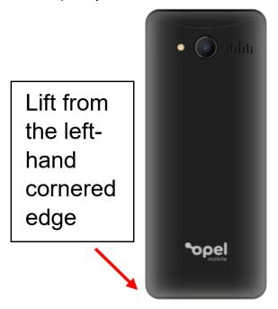
2. Remove the battery by lifting from the top first and pulling out
