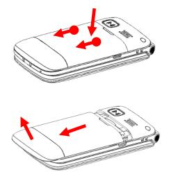
Remove the battery from the phone by lifting from the bottom and pulling out.
