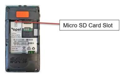
2. After you have safely placed the SIM card and memory card, **(if applicable)** in the phone, insert the supplied battery aligning the pins with the contacts, sliding down first then dropping in. Then place the back cover on correctly.
