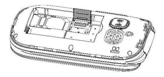
2. Insert the T-FLASH card making sure the gold contacts are facing downwards.
