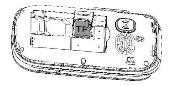
3. Then push the silver cover back down and slide to the left to lock it back into place.
