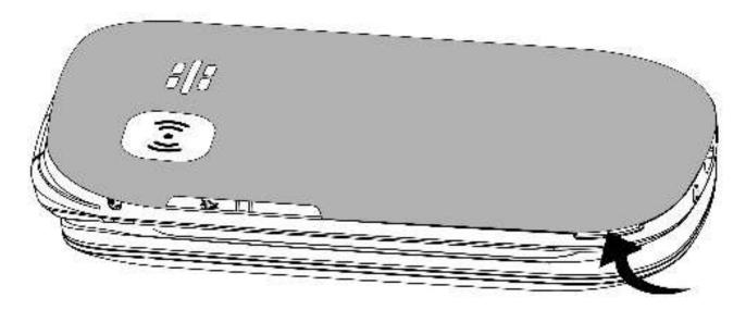
2. Remove the battery by lifting from the top first then pulling out.
