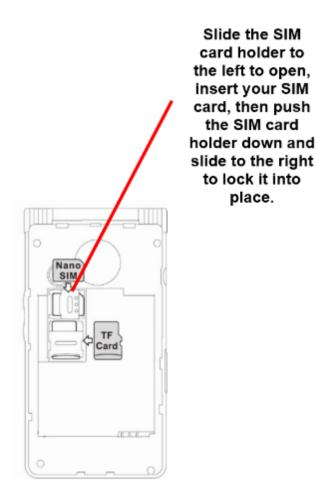
4. If you wish to use an optional Micro SD card (TF Card), using your finger, slide the TF card holder upwards to open the TF Card holder. Insert the Micro SD card into the slot. Push the TF Card holder back down and slide forwards to lock it into place. PLEASE NOTE: the maximum Micro SD size possible is 32GB.
