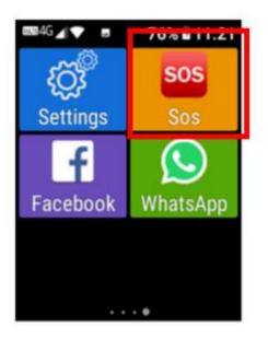
2. Once opened enable SOS mode. By clicking ok or tapping on enabled. It will show a tick symbol when it is enabled.
