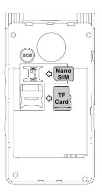
4. If you wish to use an optional Micro SD card (TF Card), using your finger, slide the TF cardholder upwards to open the TF Card holder. Insert the Micro SD card into the slot. Push the TF Card holder back down and slide downwards to lock it into place. PLEASE NOTE: the maximum Micro SD size possible is 32GB.
